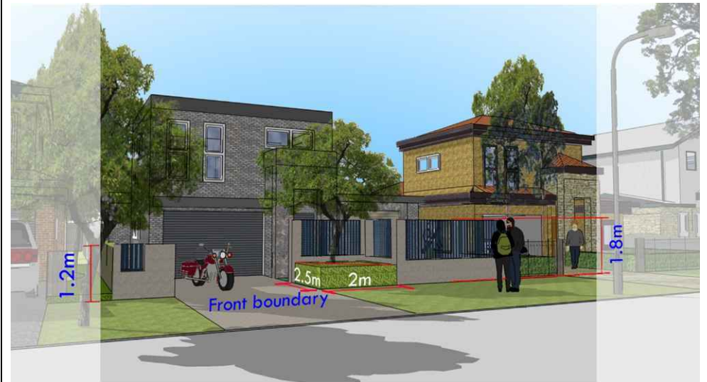
Figure D2.12: An example of a 1.8m transparent fence with landscaping complying with the driveway splay
