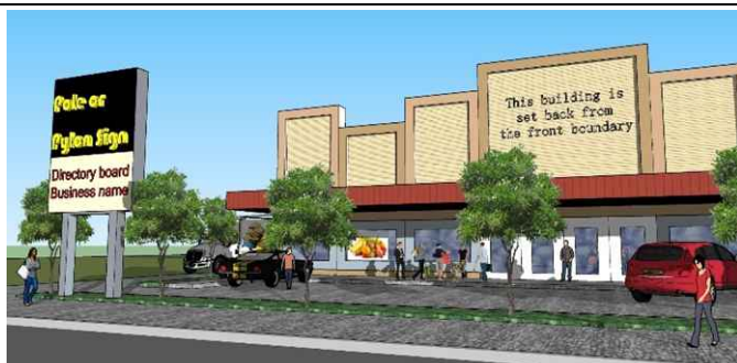
Figure C9.06: Pole or pylon signage (freestanding advertisements under 20 square metres and less than 8 meters off the ground)
